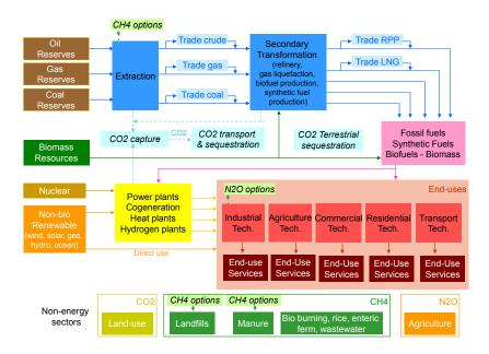
Figure 1: Reference energy system of TIAM
