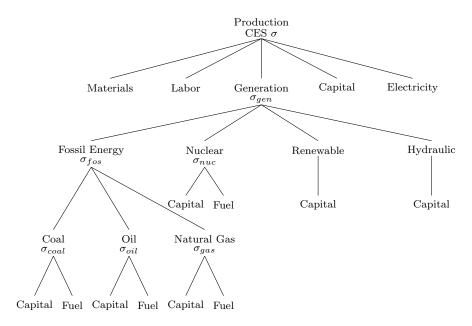
Figure 2: Nesting CES structure of electricity production
